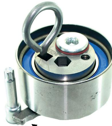
Setup screw is used to position tensioner during installation.
